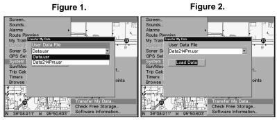
These figures show the menu sequence for loading a GPS Data File from an MMC into the unit's memory.
